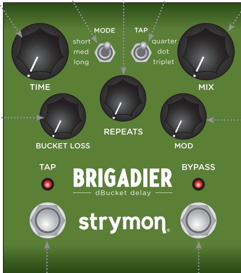
**MOD:** Adds **LFO modulation** to the delay time. Modulation is off at minimum setting. The modulation speed is slow in the first half of the knob, and fast in the second half of the knob, increasing in intensity as the knob is turned clockwise.
