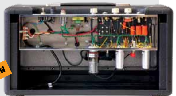
Completed Blackface Tube Reverb Kit.
