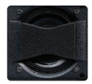
A Directivity Phase Device (DPD) on each cone driver extends the upper frequency limit for file source coupling between adjacent speakers. 6.5" drivers coherently couple as if there were twice as many 3.25" cones mounted at half the physical distance.
