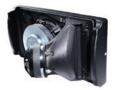
GEO M6 utilises NEXO's patented Hyperbolic Reflective Wavesource (HRW<sup>™</sup>) to control acoustic energy by creating a virtual wavesource 'outside the box', resulting in optimal wavesource coupling without destructive interference.
