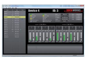
RockWorks is a real-time management system for RockNet and enhances the remote operation of complex widespread networks. Each RockNet device can be monitored and configured on screen according to the front panel operation. RockWorks enables labeling of each device and channel within the network. The software provides alarm indications and allows for a network-wide default reset of channel parameters and naming. For a more comfortable setup, RockWorks also features an offline editor.
